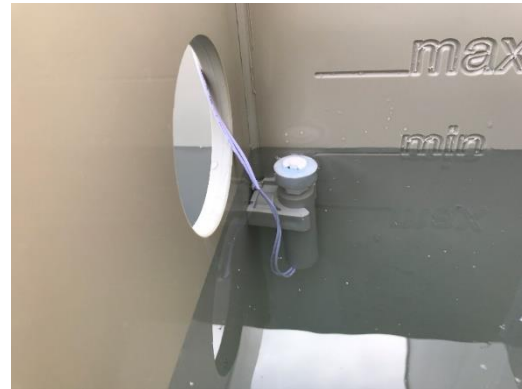
Float is in "rinse" position, pond pump is on. Drum turns and rinsing pump rinses the cloth. If the float stays in this position for 30 seconds, the electronics will go into DRY RUN MODE.
